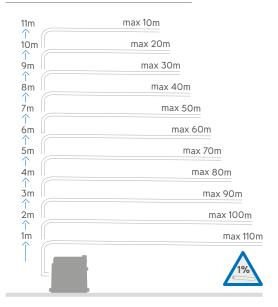
Connection to soil and vent pipe or drain
